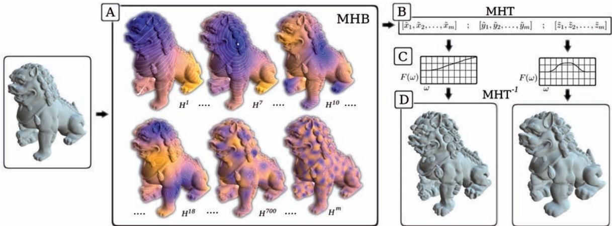
**Figure 1:** Processing pipeline of our method: A: Compute the Manifold Harmonic Basis (MHB) of the input triangulated mesh. B: Transform the geometry into frequency space by computing the Manifold Harmonic Transform (MHT). C: Apply the frequency space filter on the transformed geometry. D: Transform back into geometric space by computing the inverse MHT.
